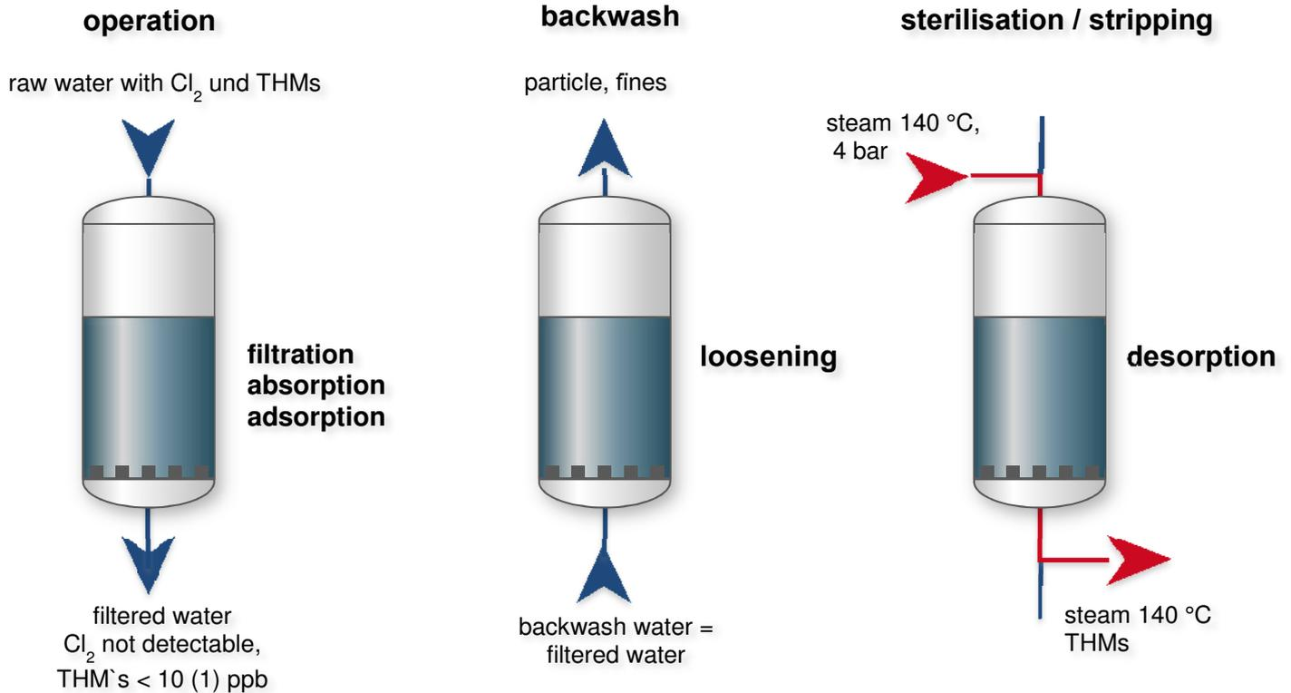
The sterilisation of an activated carbon filter should generally be done at least once a week or more often if the microbiological parameters are deteriorating. Furthermore, if the carbon filtration consists of more than one vessel, it is recommended to always operate all carbon filters in parallel. A filter should only go out of operation for sterilisation and / or backwashing, because a continuous operation is an effective way to prevent early microbiological growth on the carbon.
