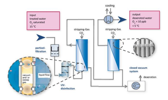
In contrast to the EROX® process, the open stripping columns are pressure less after the process and so further pumping energy must be supplied for onward transport. When using the hot process there is a risk of precipitation and with the application of an open packed column microbiology is of concern.
